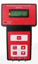
SPM-111 is a small Micro Processor based diagnostic tool for comprehensive condition analysis of rotating machinery.
